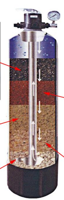
火山矿石过滤煤体(澳洲) 4 STAGE Zeolite(Australia) 有效吸附有害液体,滤除重 金属,如铅和铭等。过滤泥浆, 杂质,改善水质,增强反冲洗 It is a naturally occurring mineral rock, formed when mineral-rich underground water deposits crytalize. Its porous crystalline structure provides advanced filtration properties and possesses a unique capacity to adsorb ammonia and various ionic species(metal ions, calcium, magnesium ets).
