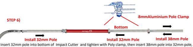
Insert 32mm pole into bottom of Impact Cutter and tighten with Poly clamp, then insert 38mm pole into 32mm pole, flexible to harvest oil palm fruit.
